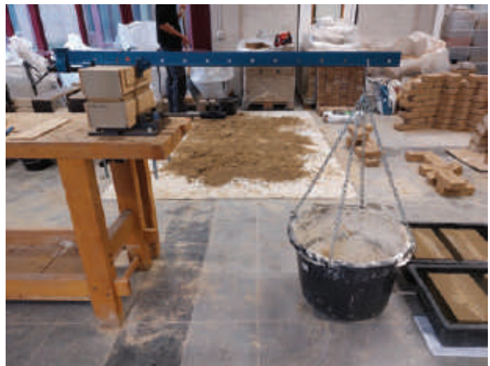
figure 2: Lab experiments on the reclaimability of earth blocks [Photo: Erik Pelicaen]
